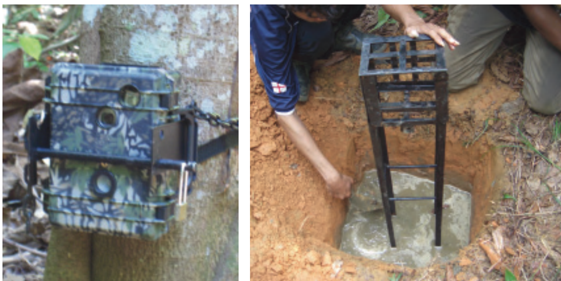
Figure 5 – A Photoscout camera-trap (left). Following persistent theft and vandalism some cameras were set up in metal cages, sunk into concrete bases (right).
